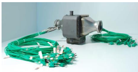
Figure 1: Functional prototype of the highly integrated TEG for use in hybrid cars.
