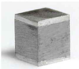
Figure 1: Photograph of Ag-Ni multi-layer metallization on SnSe thermoelectric leg
