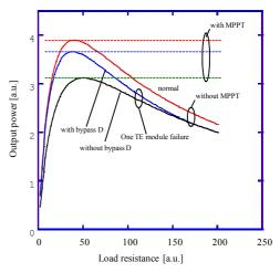
Fig.5 Effect of bypass diode on output power vs load resistance.
