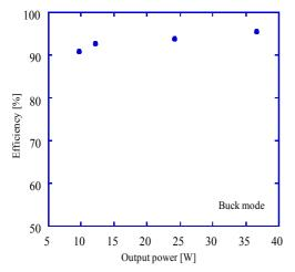
Fig.3Output power vs conversion efficiency
