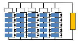
Fig.4 Schematic of electric connection of bypass diode.
