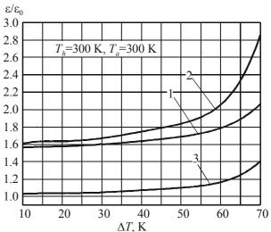
Fig. 4. Increase of coefficient of performance of permeable planar thermoelement  $\varepsilon$  of optimally homogeneous materials (dependence 1) and of functionally graded nmaterials (dependence 2) with respect to its value for nonpermeable homogeneous thermoelement  $\varepsilon_o$  fordifferent temperature differences. Dependence 3 – additional increase of coefficient of performance of permeable planar FGM thermoelement with respect to its value for permeable homogeneous thermoelement.
