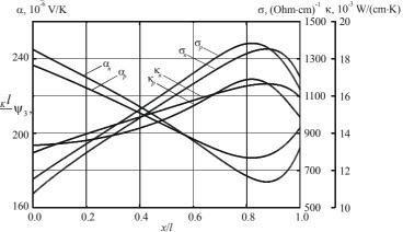
Fig. 2. Optimal distribution of material parametersalong height l of the legs of permeable planar thermoelement for temperature difference  $\Delta T=40$  K,  $T_h=300$  K (x/l – dimensionless leg coordinate).
