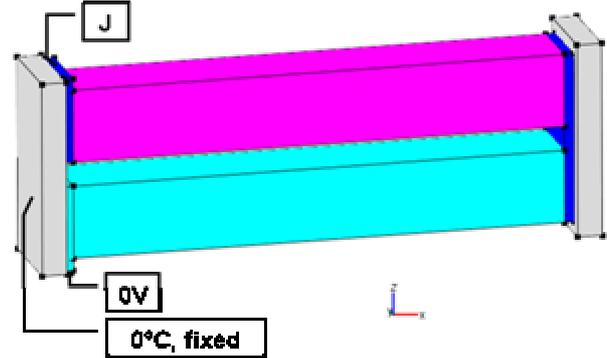
**Figure 1: The thermocouple example consists of two  $1.5 \times 1.5 \times 10 \text{ mm}^3$  legs. They are contacted with copper on a alumina substrate. The left side is kept at  $0^\circ\text{C}$  and mechanically fixed. The current density  $J$  is applied at the upper left electrode, the lower electrode is grounded.**
