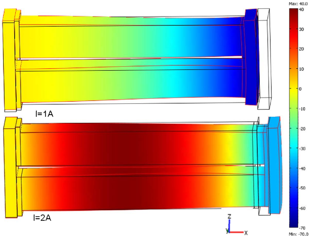
**Figure 2: The thermal expansion of the thermocouple for 1A and 2A current. The initial geometry is shown as a black wireframe, the deformed frame is red and filled with temperature coded colors. At maximum cooling near 1A, the module shrinks about 5 microns (above). At 2A, the module is thermally expanded although it is still cooling.**
