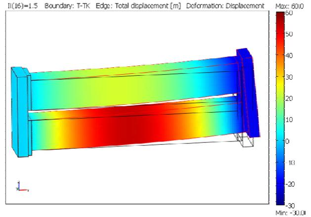
**Figure 5: A doubling of the resistivity of the lower thermoelectric leg leads to higher temperatures and thus to asymmetric thermal expansion. Other parameters like in figure 2, the current is 1.5A.**
