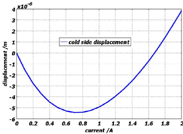
**Figure 4: thermal expansion of the module in x-direction**
