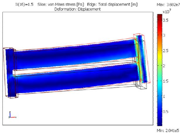
**Figure 6: Von Mises stress in the asymmetrically strained module of figure 5**
