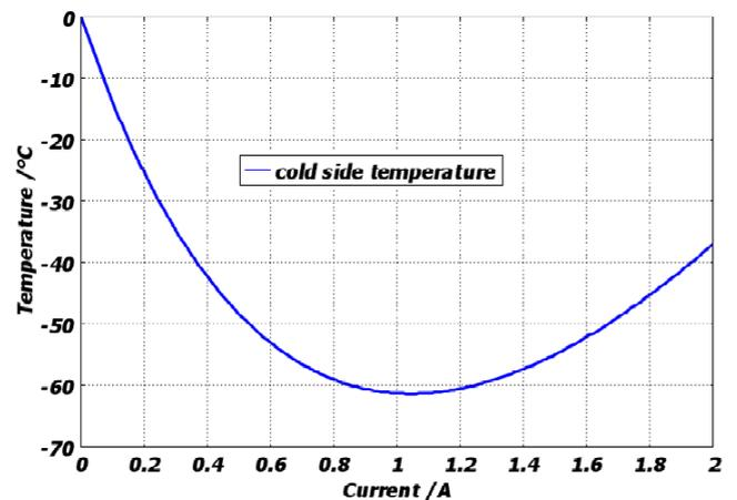
**Figure 3: The calculated cold side temperature versus current shows a**
