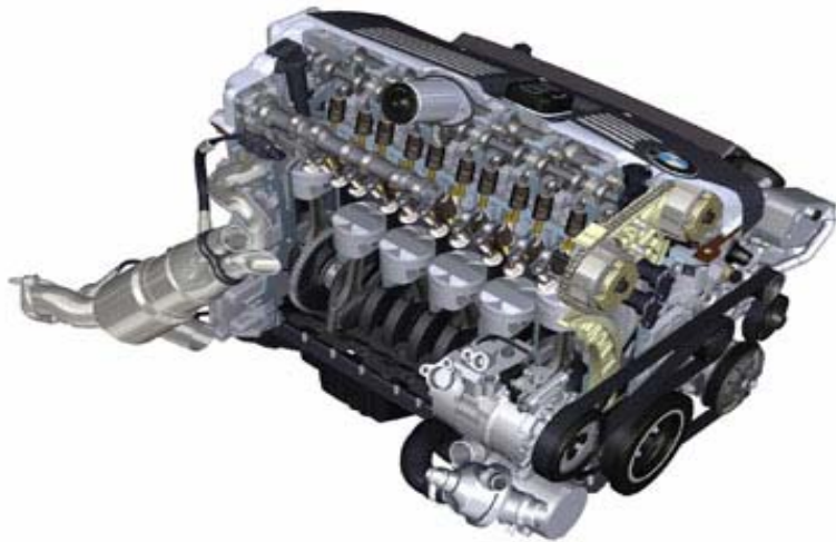
Selected engine - Inline 6 cylinder, 3.0 l displacement
