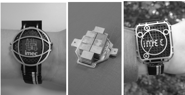
Figure 6. Wrist TEGs fabricated in 2005 for outdoor use (left) and for indoor use (right). The thermopile assembly of outdoor version is shown in the middle.
