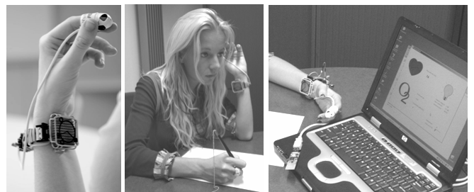
Figure 8. Body-powered pulse oximeter and the application running on a laptop with an update rate of 15 s.
