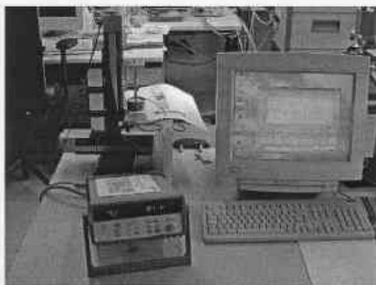
Fig. 2: Set-up of the Seebeck Microprobe. Linear stages in x-, y- and z-direction allow for a scanning of the sample. The measurement is computer controlled and fully automatized.
